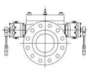
For valves size 24" and smaller, the check valve is also equipped with external counter-terbalance.
