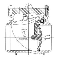
The clapper can be locked in the closed position to hold small amounts of upstream pressure for a short time; however, it is not recommended to replace gate valves as too much upstream pressure will shear the shaft keys. The external lever also serves as a clapper position indicator at all times.
