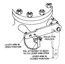
The external lever lock clapper assembly enables the user to control the clapper motion with the valve under pressure. The clapper can be locked in the open position for reverse flow or when the user wants to eliminate the clapper action.
