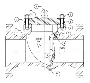
Similar in design and construction to standard swing check valves, these valves are suitable for high temperature service conditions. End flange connections can either be raised-face or ring-type joint. The metal-to-metal clapper seal together with the metal ring-joint or spiral wound cover gasket (not shown) will assure long and dependable services. Consult factory for more details.
