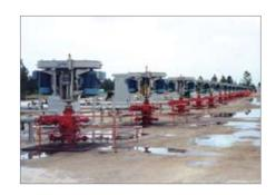
Reduced Height Saves You Time and Money The Crown CPT is approximately 50% shorter than the standard threaded components, giving easy access to the stuffing box and top drive motor mounted above the well-head.
